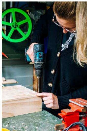
**2** Flip the box over and attach the two back pieces, side by side.
