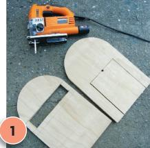
Draw identical semi-circles on the tops of two 380mm x 250mm plywood panels. Cut out with the jigsaw. Mark a mail slot about 210mm x 50mm on the front panel and a 160mm x 200mm 'door' on the back one. Cut these out. Sand rough edges.
