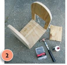
Attach the front and back panels to the base, as shown, fixing with PVA glue and galvanised nails.
