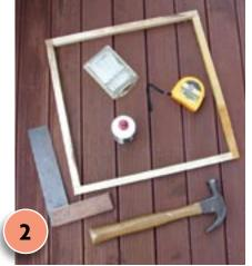
Take the four 430mm lengths of timber and join at right angles to form a square, as shown, fixing each corner with a panel pin and PVA glue. Repeat to form three more squares using the 300mm, 200mm, and 60mm lengths of timber.
