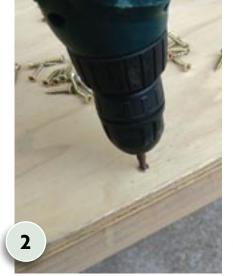
Make sure the frame is squarely aligned as you fix the plywood top to the front, back and side supports with 40mm screws and PVA glue – again, drill pilot holes first.
