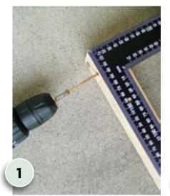
Cut timber and plywood to dimensions listed. Sand rough edges. With the setsquare as a guide, fix a table leg into the end of the front support with two 75mm screws and PVA glue (drill pilot holes first). Repeat with other legs and supports to make a four-legged frame.
