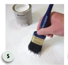
Using an old brush and stippling technique, apply one generous coat of Resene Sandtex to the table top and side edging. Allow to dry for two to three hours.
