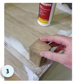
Turn upside down and fix the feet into position with PVA glue. Leave to dry overnight.
