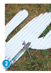
Using the pencil, draw cactus (about 110mm high) and a small circle (200mm diameter) on the mini corrugated iron panel. Cut these out with tin snips and smooth edges with a metal file. Apply a coat of Resene Galvo-Prime to both and the other two pieces of galvanised iron. Allow to dry for four hours.
