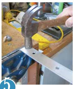
HOLD the steel pieces up against the box and mark where each section is to bend. Using a vice, bend the steel pieces, finishing off with a hammer.
