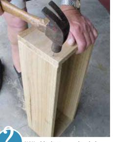
NAIL side, bottom and end pieces together to form two planter boxes. You can also use screws for greater strength.
