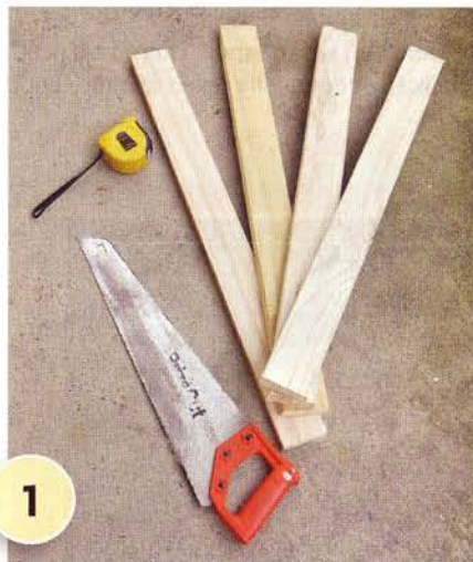
1 Measure and cut the four 900mm fence pickets to 750mm long, as shown.
