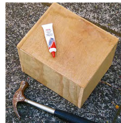
6. Using the base of the old wooden drawer, measure, mark and cut a piece to fit the back of the plywood box. Smooth rough edges with sandpaper and fix into position with PVA glue and panel pins (again, drill pilot holes first).
