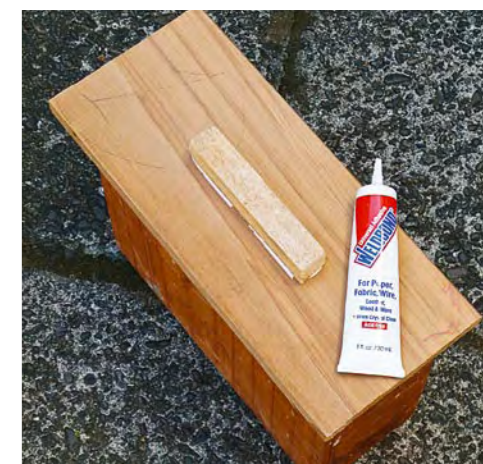
9. Cut two handles from offcuts of plywood or 10mm x 10mm timber and smooth rough edges with sandpaper. Carefully turn drawers up the other way and fix a handle to the front of each drawer with PVA. Allow glue to dry overnight.
