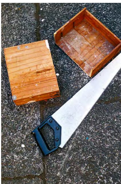
1. Measure, mark and cut the old wooden box in half, to make the insides of the two seed drawers.
