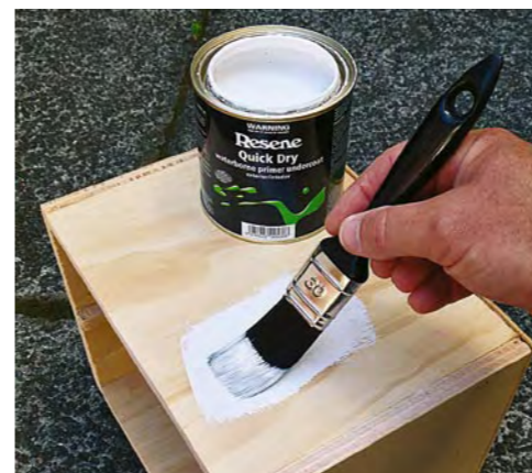
10. Paint the front and insides of each drawer and the outside and front edge of the plywood unit with one coat of Resene Quick Dry. Allow two hours to dry.
