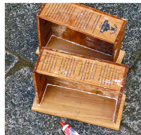
8. Slide drawers into position and then measure, mark and cut two drawer fronts from the front or sides of the old wooden drawer. Smooth rough edges with sandpaper and then glue drawers to drawer fronts with a generous amount of PVA, as shown. Allow glue to firm up.
