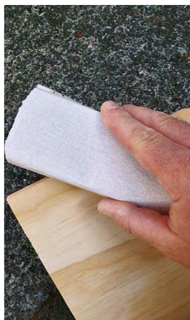
3. Smooth any rough edges on the plywood and the sawn box with sandpaper.
