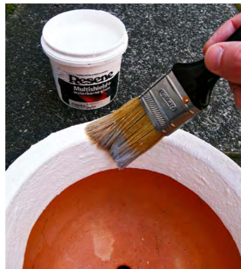
6. Apply three coats of Resene Multishield+ gloss to the rim and outer sides of the pot to create a high-gloss finish. Allow two hours for each coat to dry.
