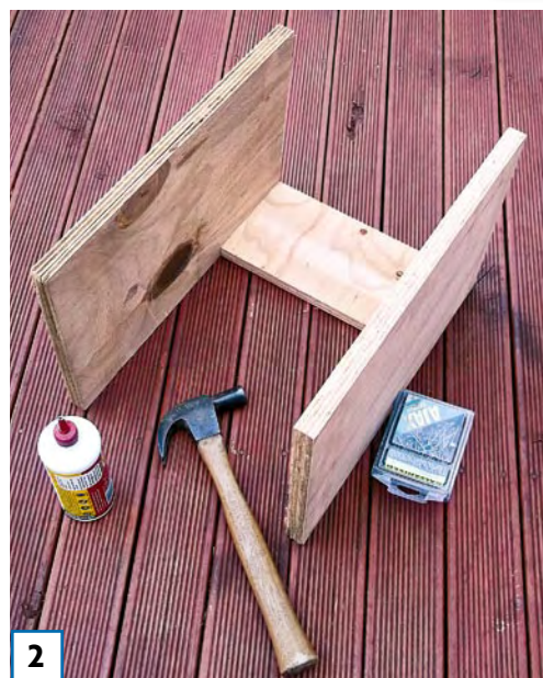
2 On a sturdy flat surface, attach the back upper section to the two side pieces, as shown, fixing with PVA glue and nails.
