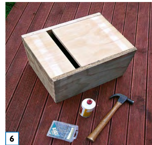
6 Fix the front lower section into position, leaving a 30mm gap, as shown. Fix with PVA glue and nails.
