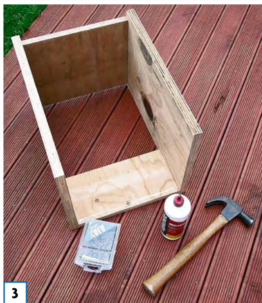
3 Attach the base to the two side pieces – the base should be positioned centrally along each side (leaving a 20mm gap at the front and back). Fix with PVA glue and nails.
