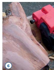
LIGHTLY sand using the belt sander, first with a coarse grade sanding belt, then with a medium grade.
