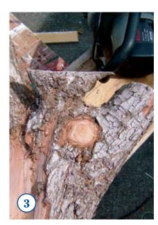
WITH a chainsaw, carefully remove any unwanted knots, lumps or small branch stumps.
