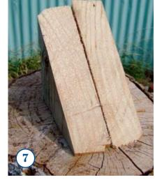
ATTACH two wedges of wood to the top of the base plinth with exterior construction adhesive - these will ensure the finished sculpture stands upright. Allow to dry.
