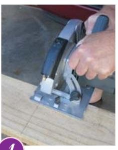
CUT timber to size. A circular or hand saw can be used, or ask your local building supplier to cut the wood to length. Sand edges with sandpaper.
