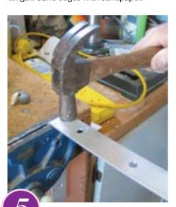
HOLD the steel pieces up against the box and mark where each section is to bend. Using a vice, bend the steel pieces, finishing off with a hammer.
