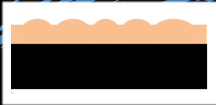
Moderate orange peel effect
