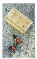
Drill six 12mm drainage holes in the base, as
