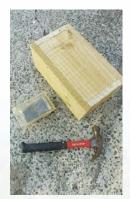
Assemble, as shown, to form a rectangular trough, fixing with PVA glue and 50mm nails. Allow glue to dry.
