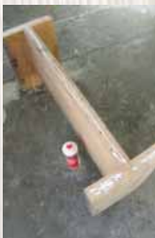
Step six Turn the bench the right way up and apply a line of PVA glue along the tops of the legs and underneath support.
