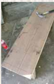
Step seven Place the seat in position and hammer through the nails, fixing to the underneath support and legs.
