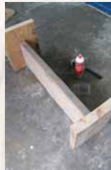
Step four Assembling the bench upside down on a flat surface, fix the legs to the underneath support using nails and PVA glue.
