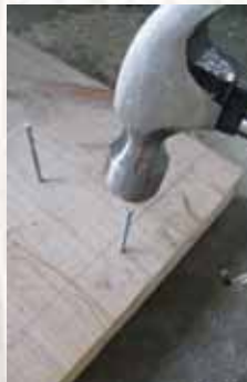
Step three Position three nails along the centre of each of the leg pieces, as shown.
