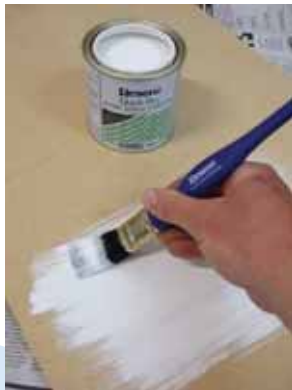
Step one Prime the piece of MDF with one coat of Resene Quick Dry. Allow to dry for about an hour.
