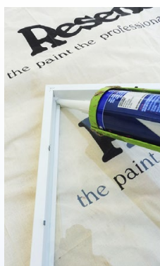
Step 3 Remove the spacers from the picture frame and apply a bead of silicon around the edge of the glass.
