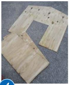
CUT the plywood to size. If you don't have a saw, some building suppliers will cut wood to exact measurements for a small fee. Sand the edges to remove any rough spots.
