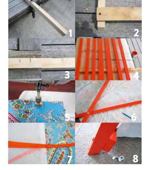
Drill a hole in the uprights 250mm from the top. Cut a 30° angle in each base.
