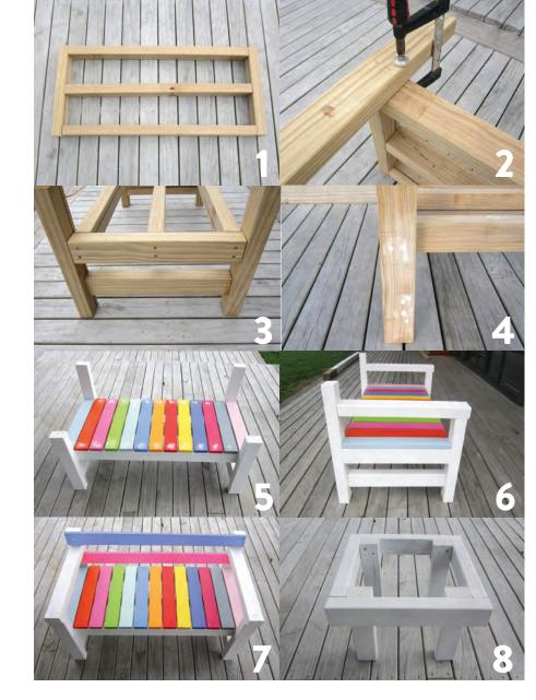
Assemble the seat as shown, making sure to countersink all screw holes and glue all joins.
