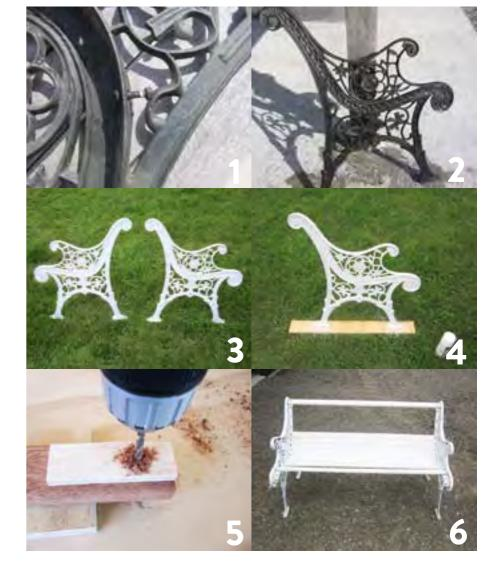
Remove all old bolts and hardware from the cast iron bench ends. You can try CRC or a similar product or use the hacksaw to cut through the bolts.
