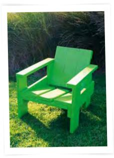
To make the legs, place 1 x 450mm length at each end (one above and one below) of a 650mm length (140mm x 32mm dimensions) to form an overlapping H shape. Drill and screw together with 50mm screws. Repeat to make the other set of legs.
