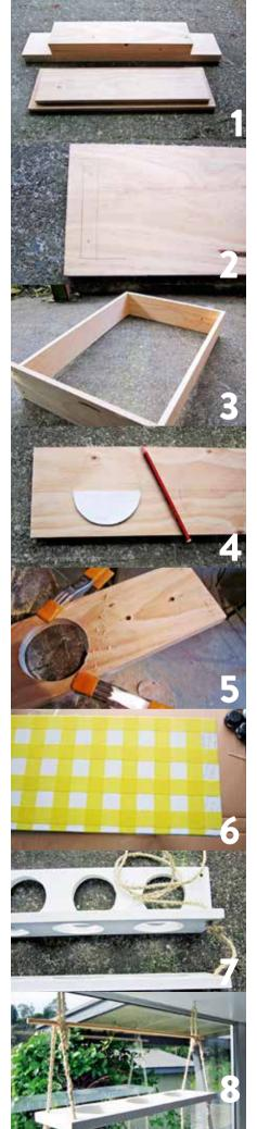
Cut the timber to length. Mark, drill and countersink two holes at each end of the top board, 45mm in from each side and 10mm in from the edge.
