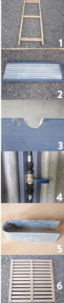
Mark side bars so the top strut forms the top of the frame, the second placed flat directly below it and the following two with a 865mm gap between leaving a gap at the bottom (see photo). Drill screw holes, countersink and screw struts into position using the 65mm screws. Repeat for second panel. Sand and apply 2 coats of a suitable paint (I used the Resene Waterborne Woodsman stain 'Skywater').
