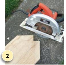
Cut out the plywood pieces with a circular saw and smooth rough edges with sandpaper. When cutting out one side of the awning, the saw blade will need to be set at 45° so it slopes down when attached.
