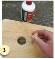
Drill a few 12mm holes in the base, then a central 12mm hole 100mm up from the bottom of the front wall and lastly, a 40mm hole 20mm above this. Insert and glue the dowel in the smaller hole.
