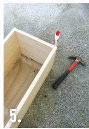
Measure, mark and cut the 280mm x 20mm timber into two lengths measuring 925mm and two lengths measuring 250mm. Smooth any rough edges with sandpaper.
