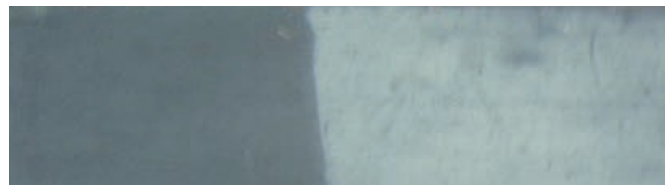
Resene Paint Prep and Housewash has successfully 'de-chalked' the left hand side of this heavily oxidised panel.
