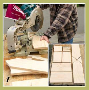
Cut out the pieces for the birdhouse, using the full plank width. The 180mm x 270mm roof pieces have a 45-degree bevel on one long edge so they fit together to form a gable. Ours is made for starlings so measures 450mm high to the top of the gable, with 360mm high sides. The base measures 180mm x 140mm. Sand any rough edges or surfaces.
