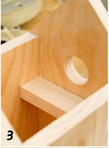
Mark the hole in the centre of the front panel. Line the top up with the 45-degree gable angle. Drill a hole for the peg. Also drill a couple of drainage holes in the base piece of the birdhouse.
