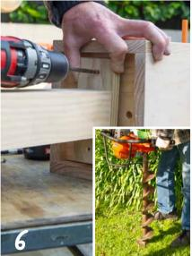
Attach the platform to the top of the pole. Bore or dig a hole and set the pole with quick-set concrete. Fill half of the birdhouse with dry wood shavings, moss or pine needles to give the birds a nesting start.
